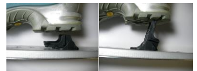
The heel riser mounted to the ski in the correct position (above left). The heel riser flipped up for easier climbing (above right).
