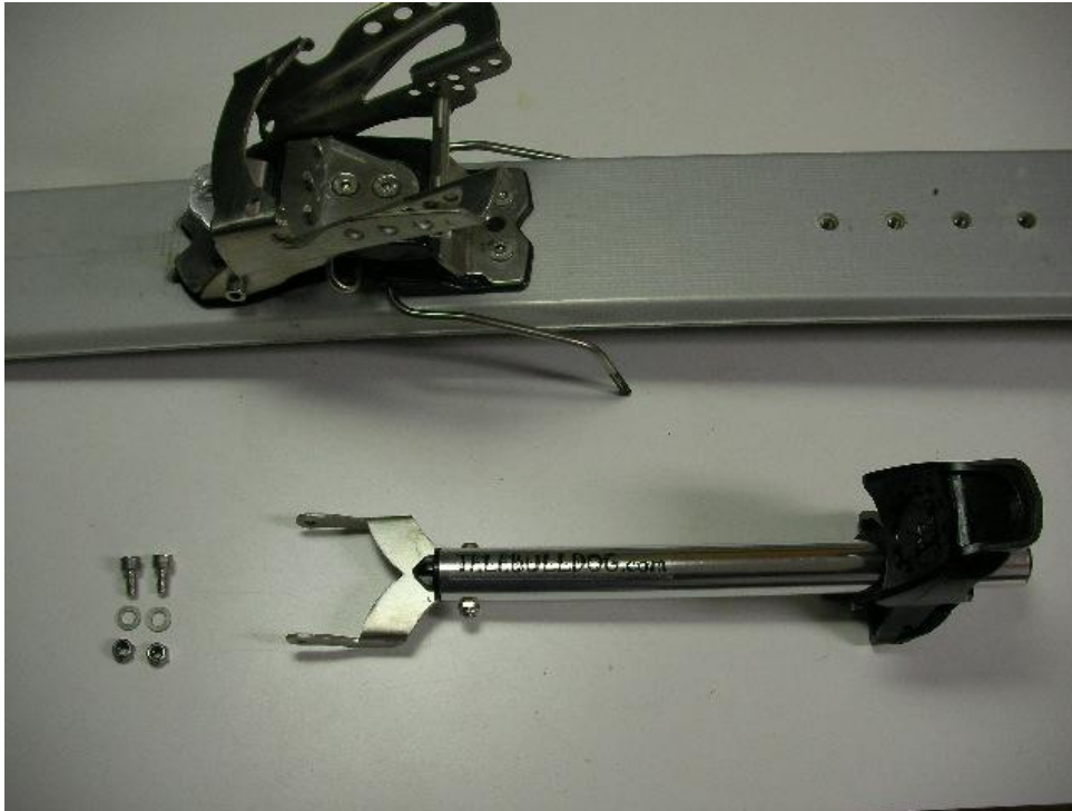
Picture above shows the parts needed to secure heel attachment to the toe piece.
