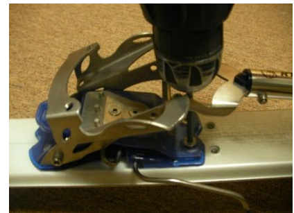
Mount the bindings with the rear mounting holes first
