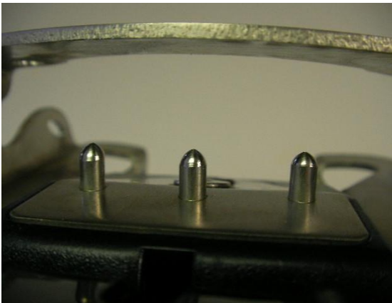
LiteDogz and classic Telebulldog bindings have longer pins that align with pin holes in the ski boot and hold the boot in the binding without the heel attachment.
