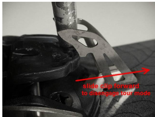
To disengage tour mode, do the opposite steps: 1) keep your boot in the binding 2) use a ski pole to depress the toggle 3) slide the tour clip forward while lifting the heel of the ski boot slightly.
