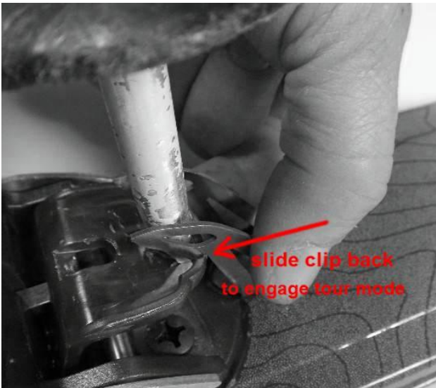
Then, press down on the toggle using a ski pole and slide the clip back using your fingers...
