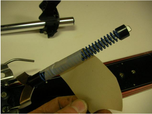
The spring is wrapped with a Teflon tape to prevent friction and squeaking inside the tube.
