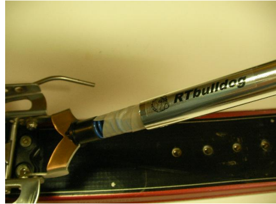
Slide tube back on and replace bolt when you are finished adjusting the spring.
