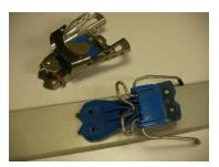
Step 2) remove ski brake wire and replace it into new plastic
