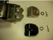
push latch forward with your thumb and drop new cotter pin into the hole at the end of the latch
