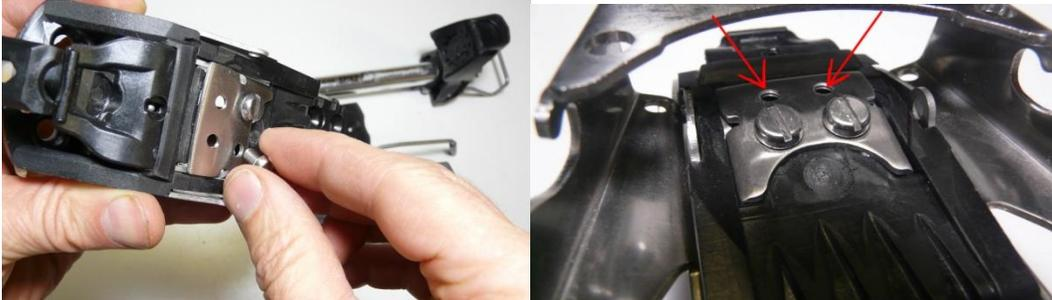
The screws in the top surface of the ski brake activator provide a raised contact point with the sole of the boot for tight fit. The screws can be removed for easier step-in action, or raised for tighter contact with the boot. There are 4 threaded holes in the pivoting plate. The 2 rear screws are recommended and installed. Two additional screws can be added to the front of the pivoting plate for more active feel.
