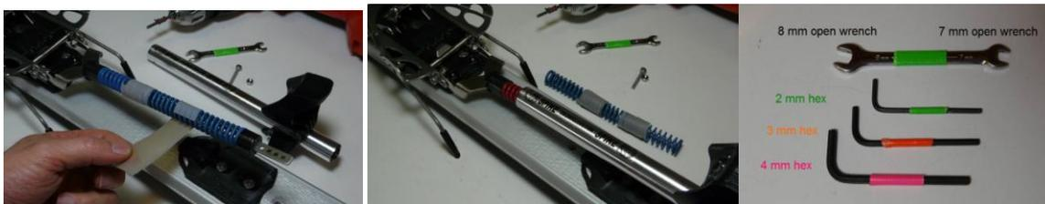
The springs are covered with a teflon tape for smoother action. Right photo shows the tools needed to work on the SPIKE bindings.
