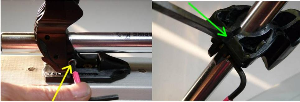
use a 4 mm hex wrench and loosen the bottom bracket screw (yellow arrow above), then use screw driver to spread the bottom bracket (green arrow above). Slide the heel throw forward or back along the tube.
