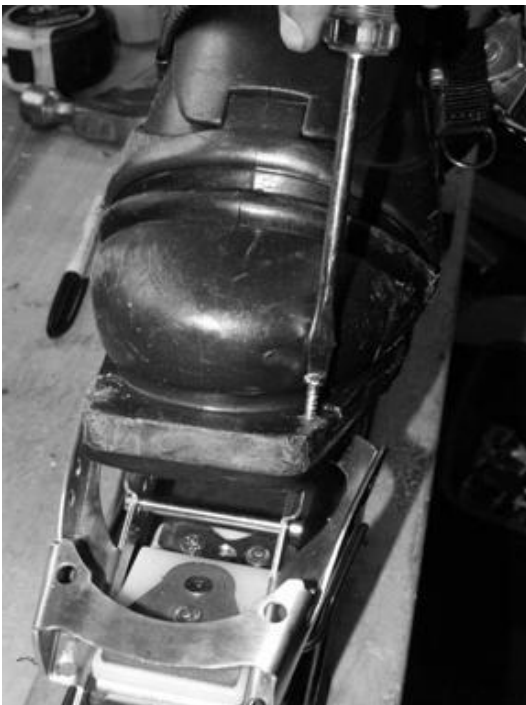
Figure 3 Remove boot from binding and screw into tap holes, 3/4" #8 stainless steel wood screw.
