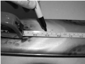
Alternatively, balance the ski on a sharp edge and mark the balance point on the ski.
