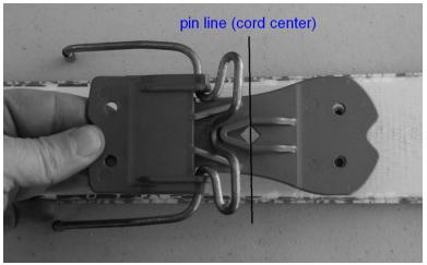
Place the mounting template over the ski and line up the center point mark on the ski with the 'pin line' on the template.
