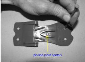
Mark the four mounting holes with a sharp point. Again, make sure that the long axis of the template is parallel to the ski.
